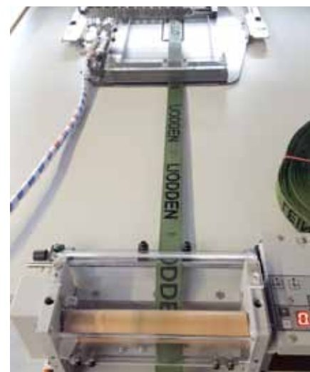
ROLL2BASKET device for embroidering on textile band
