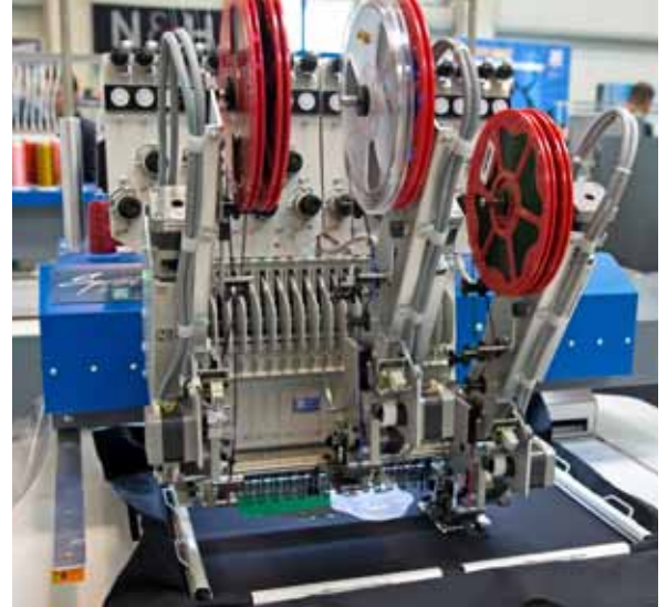
A SPRINT 7 with a triple combination of ZSK's Twin Sequin Device offering 6 different sequins.
