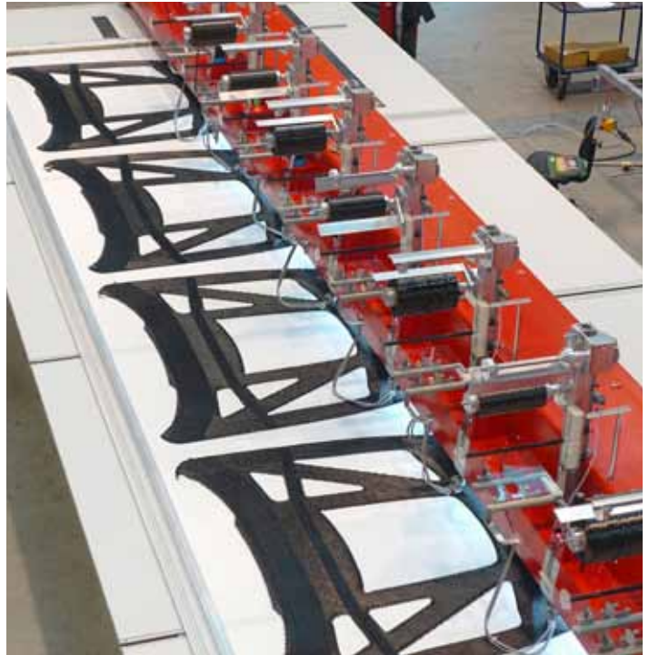
Initial designs developed on low cost single head prototyping machines can quickly be scaled to production machines for an automated additive manufacturing process.
