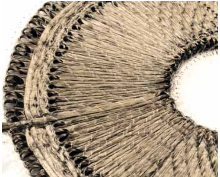
Dry carbon fiber preform created by TFP allows for control of radial and curvilinear reinforcement.
