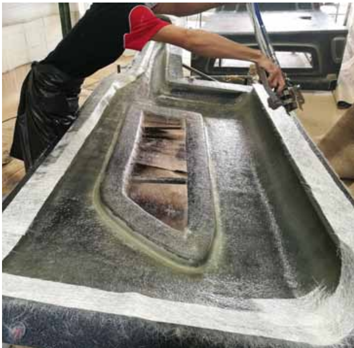
A worker sprays chopped fiberglass into the resin stream for fast composite construction. However, the resulting mechanical properties are less controlled and optimized when compared with TFP on medium to small geometry parts.
