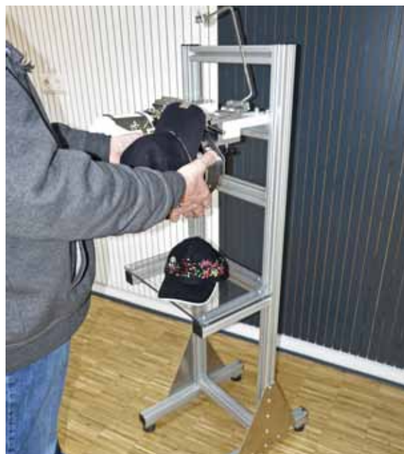
The Cap Framing Station can be adjusted to a comfortable and healthy height for your operator to avoid causes for back pain.
