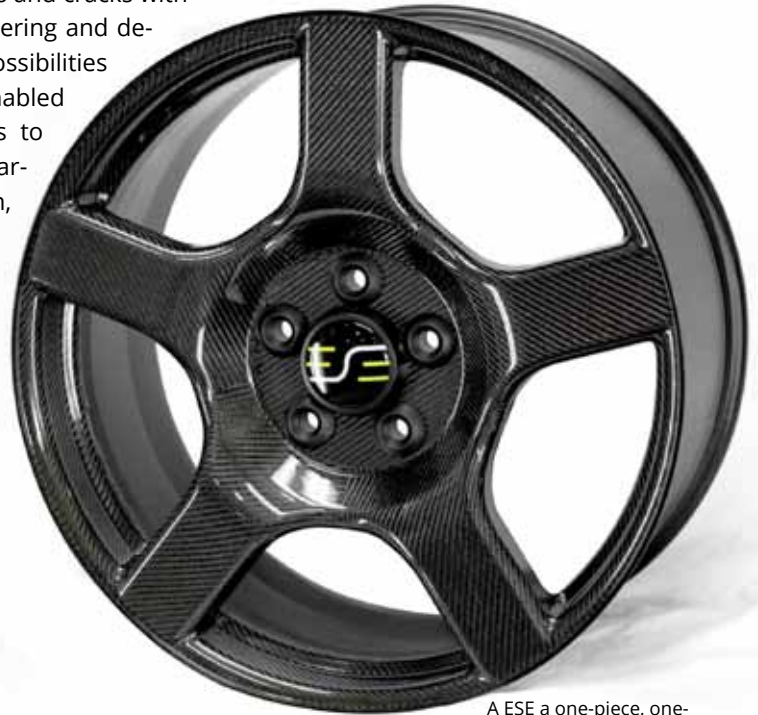
A ESE a one-piece, one-cure, carbon fibre wheel
