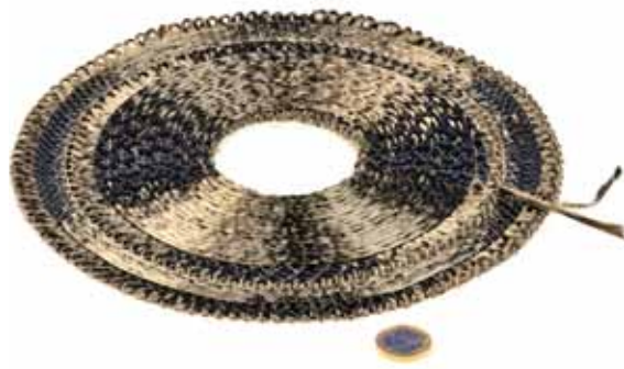
Unlike many tape laying systems, TFP allows for circular reinforcement to easily be integrated into a composite part.
