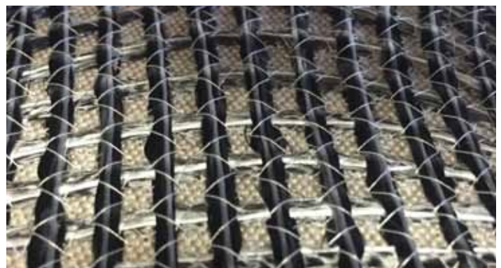
Multiple materials can be stitched into the same preform in patterns that can tailor stiffness, drapability, and other mechanical properties.
