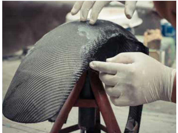
A worker completes a composite layup for a small sized complex geometry. While the infrastructure cost is initially less, success for this technique is dependent on the skill of the labor.
