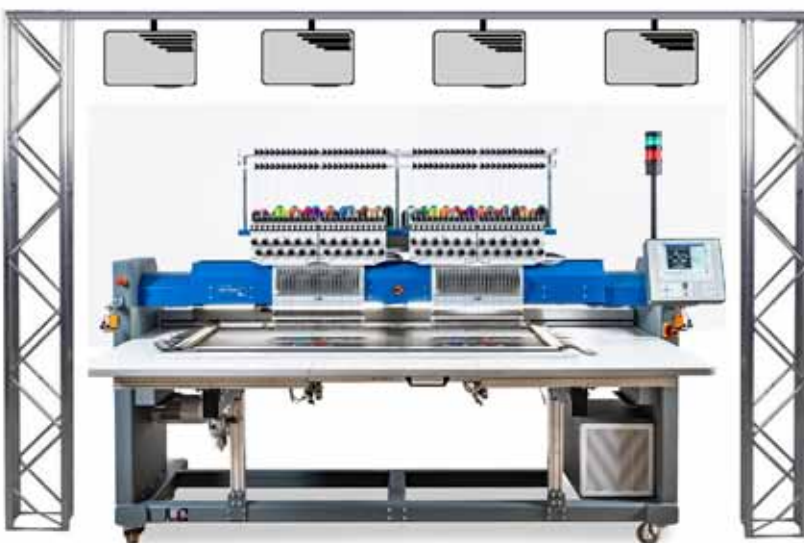
Projectors installed on a bridge over the embroidery machine.
