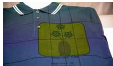
Frame turn yellow when design does not fit into the defined frame
