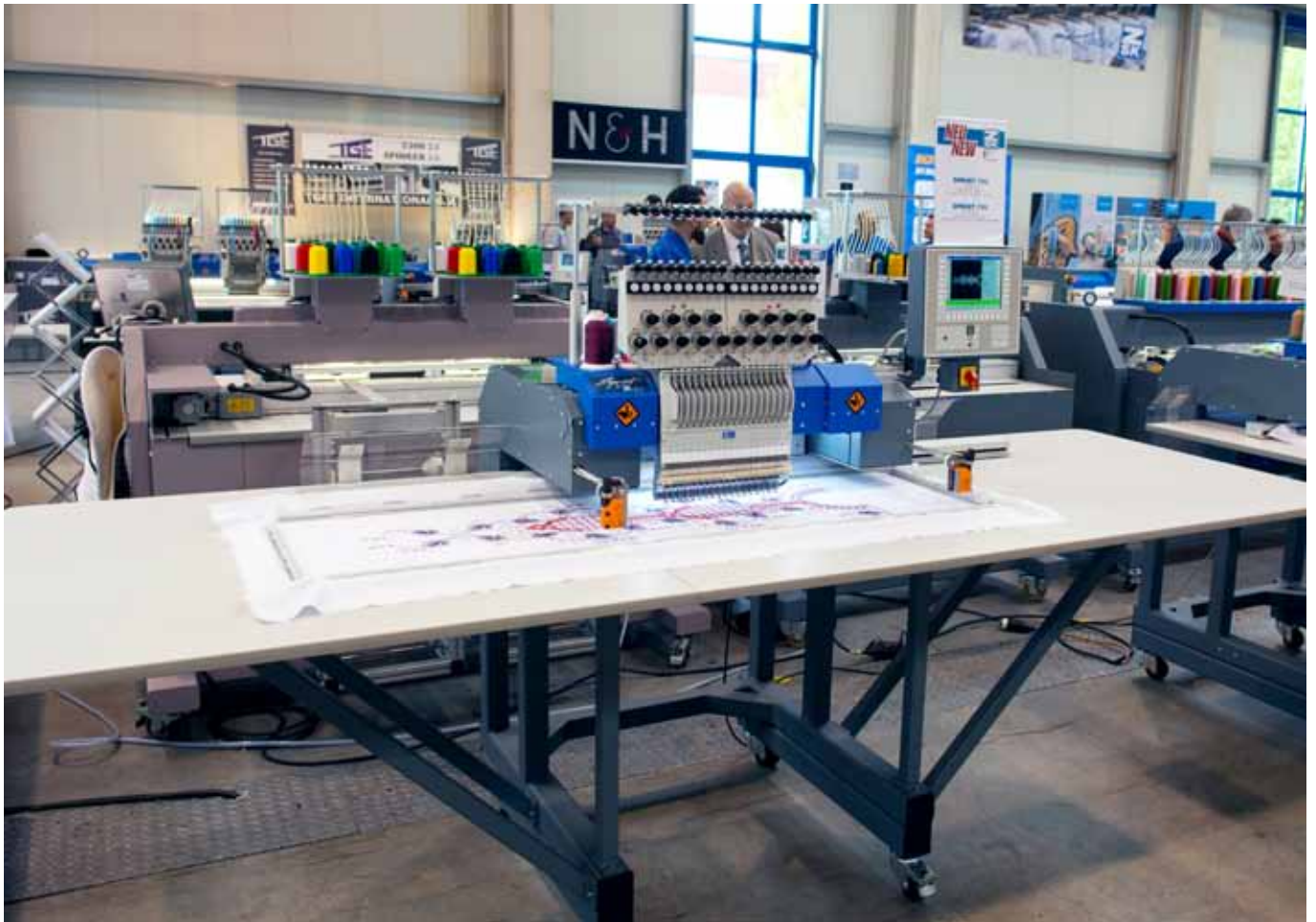
ZSK STICKMASCHINEN new SPRINT 7XL with an max. embroidery field of 1.400 mm width and 400 mm depth.
