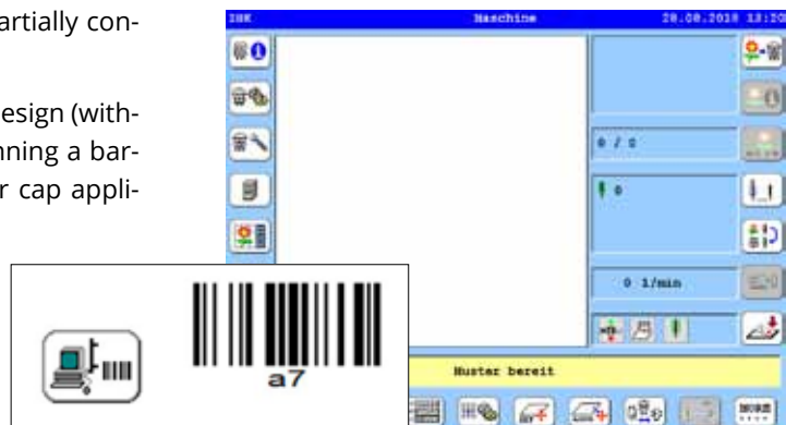
Supports design loading via network thru barcode functions
