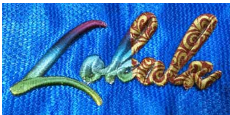
Figure: No Display Error: Printed on transfer paper, colours can be fixed onto embroidery via heat press.
