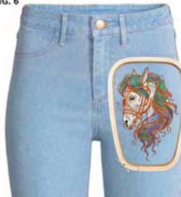
FIG. 6 – Special trapezoid-shaped frame provides optimum sewing area in the upper thigh section of a pant.
