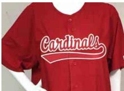
Since there is an overlap of material, the design cannot be split in half. Instead, the design must be divided into two sides that have overlapping sections in the middle.
