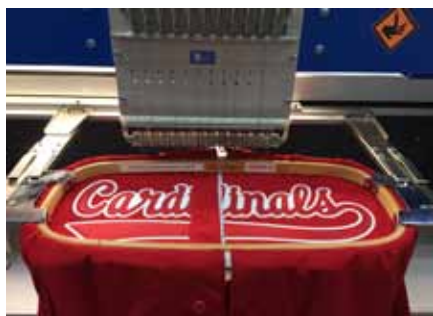
Before applying the hoop, lay out the proof on the jersey, and confirm that it will not stitch over any buttons.
