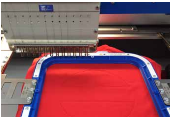
The first step of the process is typically a running stitch that follows the exact size and shape of the appliqué design.
