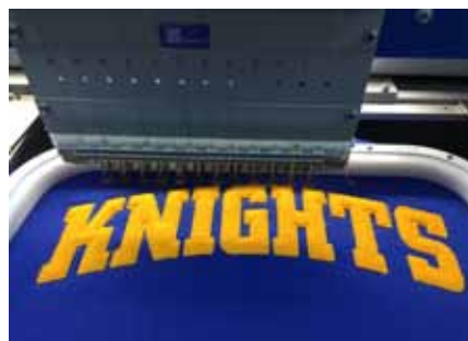
The tack-down stitch runs just a bit to the inside of the appliqué fabric to hold it in place on the garment and gives the operator a chance to inspect the appliqué before the cover stitch.
