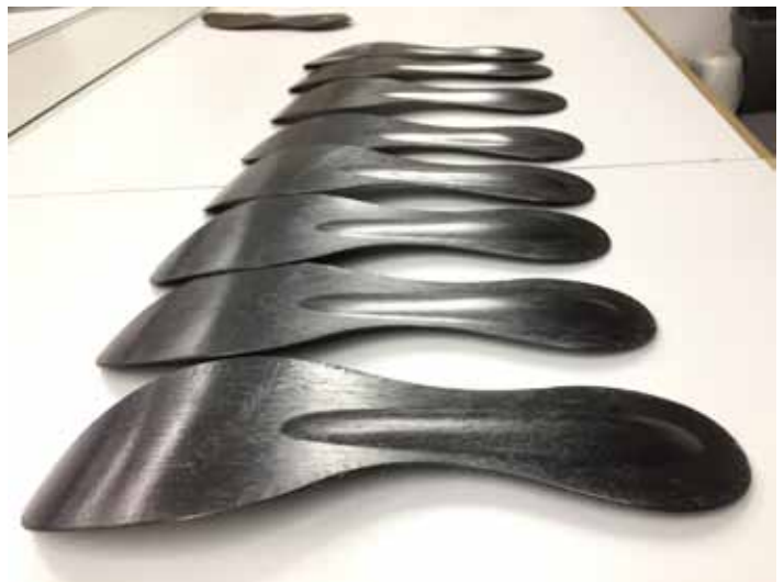
Fig. 2: The moulded preforms, after a compression moulding cycle of under 3 minutes.
