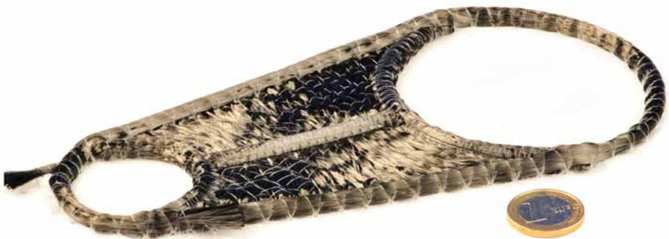
Figure 1: Thickness is built around the perimeter and in the center of the part above. This additional thickness allows the part to better resist an applied bending moment while reducing material cost by not reinforcing areas that do not require additional support. Additionally, curvilinear placement of carbon around the holes helps to minimize crack propagation often seen in orthogonal woven sheet laminate design while also reducing potential post processing and waste material.
