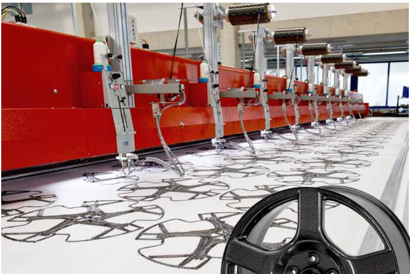
Fig. 3: ZSK Technical Embroidery System CZCW 0800-900D creating wheel reinforcement preforms
