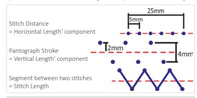
Figure 6 – Parameters to determine the ZigZag Stitches
