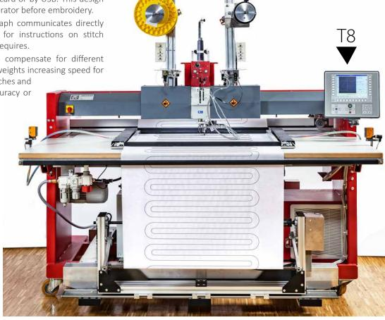
Figure 3 – T8 Control Unit at a JGW 0100
