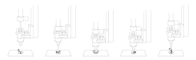
Figure 13 — shows the process of making a Chenille Stitch. This stitching process rapidly proceeds over 12 times/sec.
