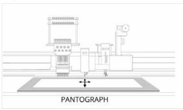
Figure 2 – The Pantograph moves in x and y directions.
