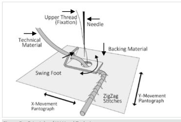
Figure 5 – Principle of W-Head Technique
