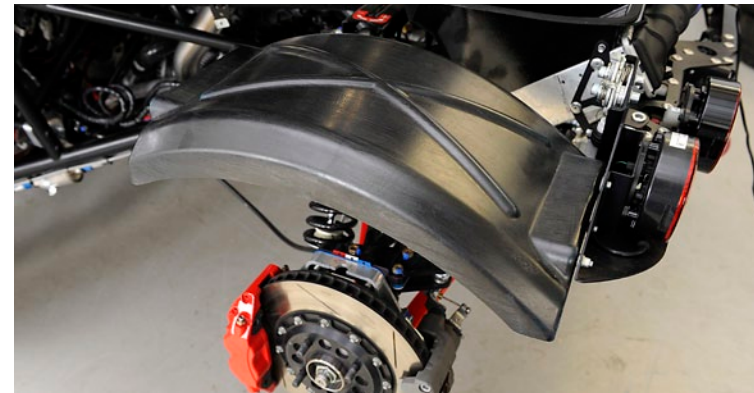
Fig.: Inner wheelarch constructed as TFP component manufactured by SHAPE for the Elemental Motor Company
