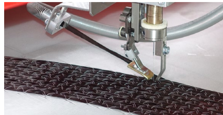
Fig.: ZSK W-Head: Embroidery Technology to lay fibres, wires and tubes.
