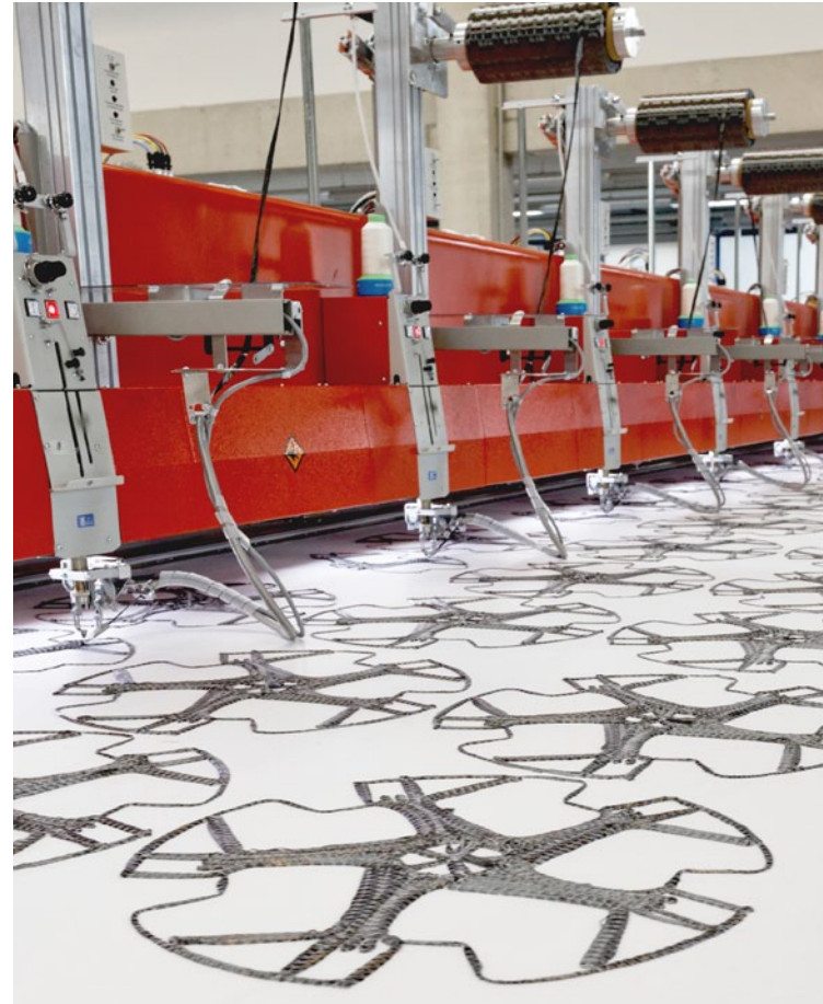
Fig.: ZSK Technical Embroidery Systems increase the speed, reliability and scalability of the process to bring composites to the mainstream.
