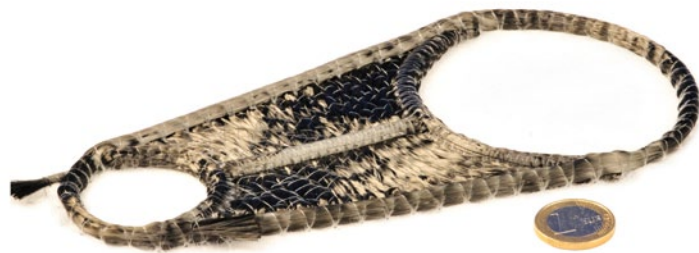
Fig.1: Carbon preform with additional thickness and curvilinear placement of carbon around the holes.
