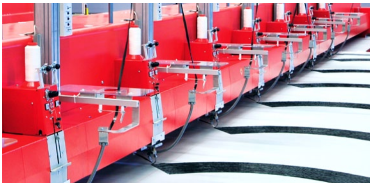
Fig.: ZSK Technical Embroidery System with up to 15 laying heads.
